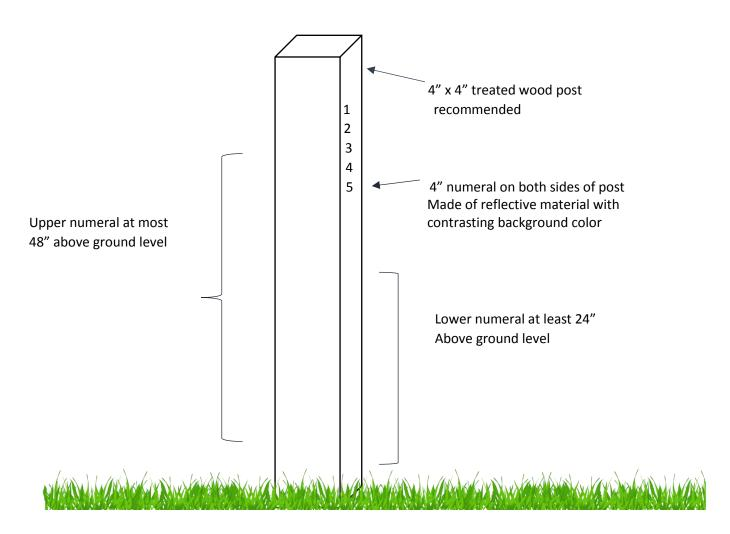
A POST SHALL BE LOCATED NOT MORE THAN 20 FEET FROM THE ROAD RIGHT OF WAY AND NOT MORE THAN 10 FEET FROM THE VEHICULAR ENTRANCE OR DRIVE TO THE PRINCIPLE BUILDING
